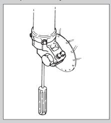
1. The compression adjuster is located at the bottom of the fork leg.
