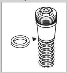
3. Spring preload is adjusted with washers and optional springs are available.
